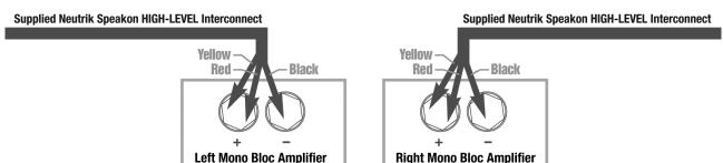
yellow wire from the twisted pair. This will reduce output by half and restore a natural dynamic. If the amplifier is of balanced differential design, please follow the instructions in the section above labeled Differential Connection.
