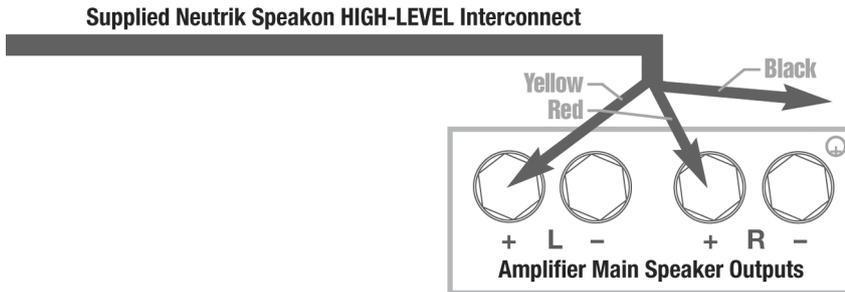
**NOTE:** The Serie S-SHO models are equipped with internal circuitry to allow seamless connection to Class-D (digital) amplifiers. If connecting to a Class-D amplifier, follow the above connection procedure for differential amplifiers.
