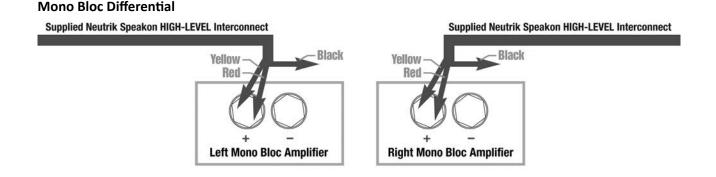
• If connecting a single REL as a dedicated centre channel sub, an insider tip is to consider connecting to the rear of the speaker, rather than routing the REL High-Level enable all the way back to the amplifier. Connect the black wire of the REL to the negative centre channel speaker terminal; twist together the red and yellow wires and connect this paired cable (red/yellow paired together) to the positive centre channel speaker terminal.
