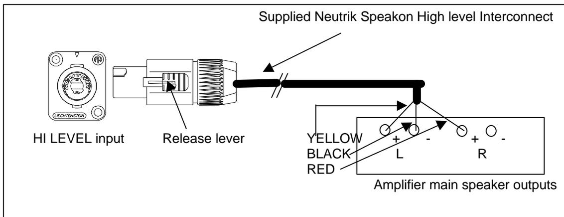
**High Level connections should be made to the same binding posts as the main speakers**
