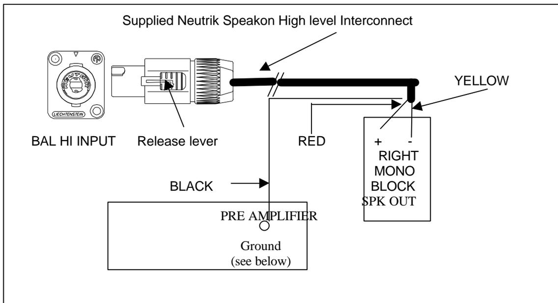
High Level connections should be made to the same binding posts as the main speakers
