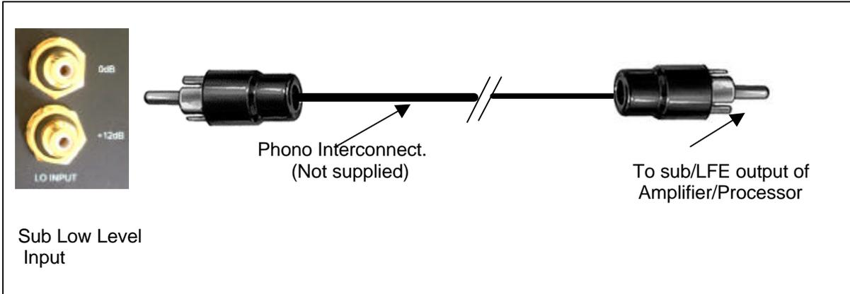
Two low level inputs are provided, 0dB and +12dB, Connect as shown above using a phono to phono interconnect (not supplied). Plug one end into the sub/LFE output on the amplifier/processor and the other end into the 0dB input on the sub woofer. If when using the 0dB input the output of the sub woofer is too low then use the +12dB input.
