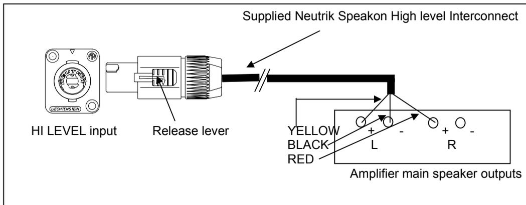
High Level connections should be made to the same binding posts as the main speakers. Connect as shown above. Red to the amplifier’s primary right speaker red terminal, yellow to the amplifier’s primary left speaker red terminal and black to one of amplifier’s primary speaker black terminals (not both).
