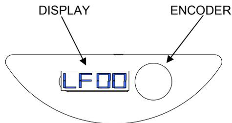
All the functions shown on page 9 and 10 are available via the remote control and the encoder on the front control panel.
