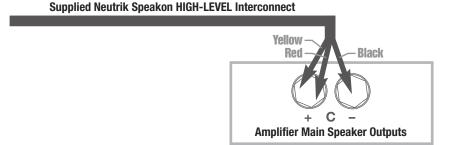
• If connecting a REL as a dedicated rear channel sub, connect the black wire of the REL to either the left rear or right rear negative speaker terminal; connect the yellow wire to the left rear positive speaker terminal; connect the red wire to the right rear positive speaker terminal.
