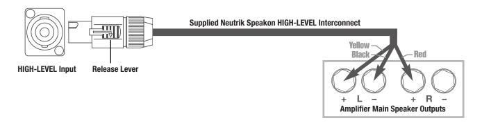
• For differential (i.e. fully balanced) amplifiers using one REL, simply use the standard connecting scheme with the exception of connecting the black wire to chassis ground (i.e. a metal bolt or screw, preferably not painted or anodized, on the chassis of the power amp or receiver), not to a negative speaker terminal, and then connecting into the HIGH-LEVEL input on the REL. Please contact your dealer should there be any questions concerning this or any other hookup procedure.
