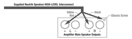
**NOTE:** The Serie T models are equipped with internal circuitry to allow seamless connection to Class-D (digital) main amplifiers. If connecting to a Class-D amplifier, follow the above connection procedure for differential amplifiers.
