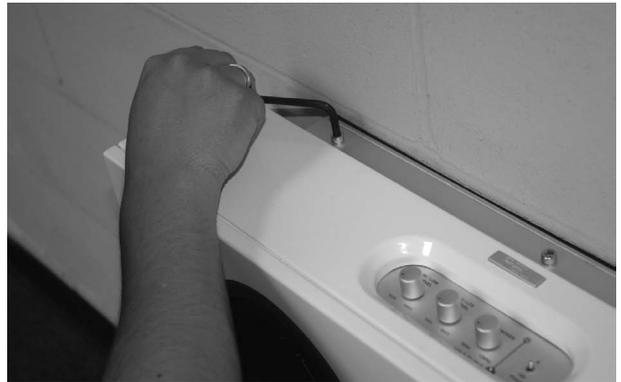
21 The fit will be snug. Draw the cabinet into place using the three 13.5mm long cap head top mounting hardware. Tighten the three provided screws 1/2 turn at a time starting with one side and rotating through each one. Tighten the three provided screws 1/2 turn at a time starting with one side and rotating through each one. Using this method will take several passes to get the screws tight. You will notice that with each pass the Habitat1 is evenly pulled into the bracket.
